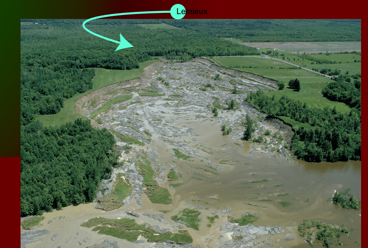
1993 Lemieux Landslide was a rapid earthflow in Leda Clay. The town of Lemieux was moved prior to the Leda clay landslide.
